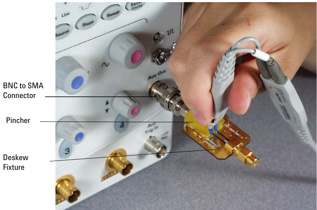
Figure 60 Browser Probe Head Calibration Connection Example
